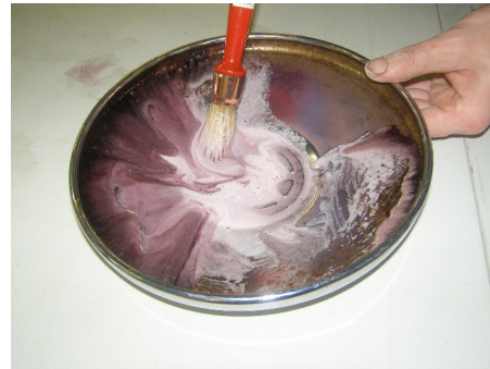
WORK INTO THE RUST
